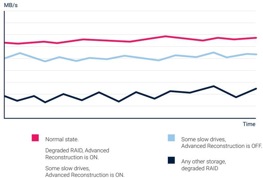
Skipped data recovers from RAID checksums. Due to the proprietary RAID engine, checksum calculations takes less time than common read operations from an average physical drive. Therefore, total array performance stays high and stable.
